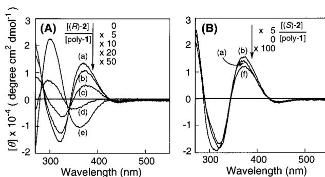
**Figure 1.** CD spectral changes of poly-1 with (*R*)-2 (A) and (*S*)-2 (B) in DMSO; the molar ratio of 2 to monomer units of poly-1 is 0 (a), 5 (b), 10 (c), 20 (d), 50 (e), and 100 (f). The CD spectra were measured in DMSO solutions in a 0.05-cm quartz cell at ambient temperature (*ca.*, 20–22 °C) with a poly-1 concentration of 1.0 mg (3.9 mmol monomer units)/mL.
